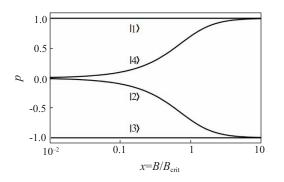
Fig. 4 The nuclear polarization  $\left(p = \frac{n_{\uparrow} - n_{\downarrow}}{n_{\uparrow} + n_{\downarrow}}\right)$  of each Zeeman state. Here  $n_{\uparrow}$  and  $n_{\downarrow}$  denote the number of particles with spin up and down.
