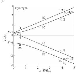
Fig. 3 The Breit-Rabi diagram of the hydrogen atom. The magnetic field and the energy are normalized by the critic field  $B_{\rm crit} = 50.7$  mT and the hyperfine splitting energy  $\Delta E = 5.87 \times 10^{-6}$  eV.
