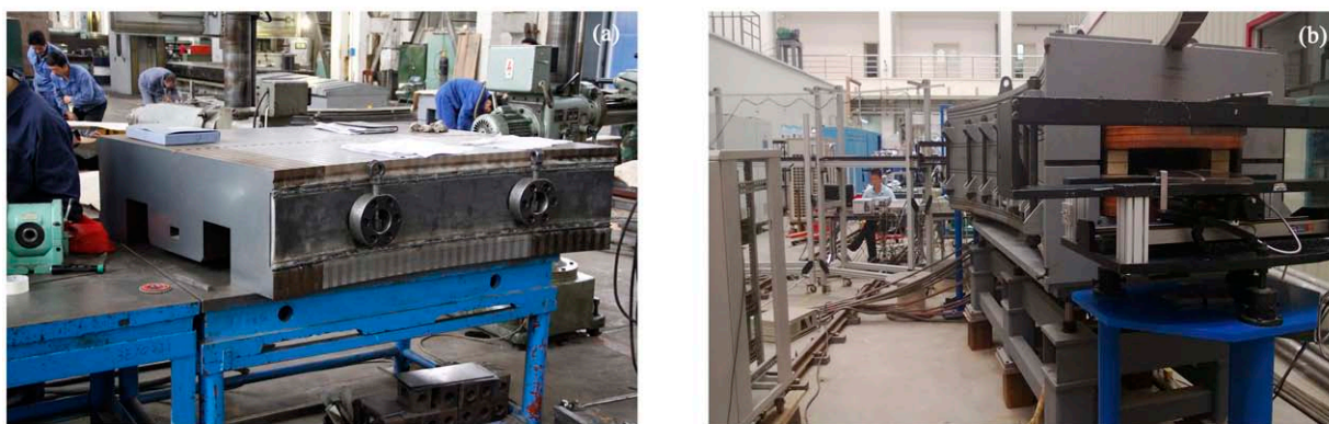
Fig. 2 (color online) The fabricated quarter lamination steel and the first dipole of HIMM.
