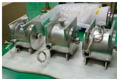
Fig. 6 (color online) Superconducting solenoid of C-ADS injector-II with helium vessel.
