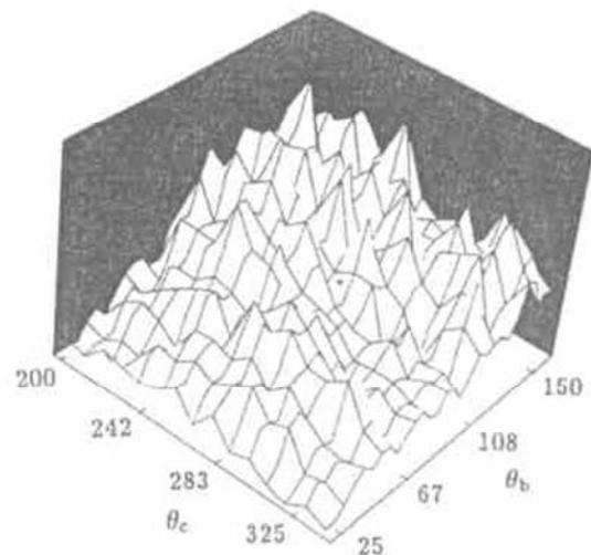
Fig. 1 Three-dimensional plot of the measured, relative 5DCS for DI of Ar<sup>2+</sup> (3p<sup>-2</sup>), plotted versus both ejection angles  $\theta_b$  and  $\theta_c$ . Kinematical parameters are:  $E_0=561.4$  eV,  $E_a=500$  eV,  $E_b=E_c=9$  eV,  $\theta_a=+1.5^\circ$ ,  $k=0.4$  (atomic unit),  $\theta_K=336^\circ$ .
