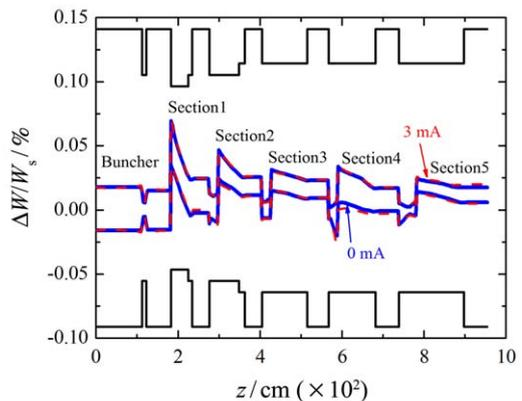
Fig. 8 (color online) Energy spread for 98% of the particle along IH Structure.
