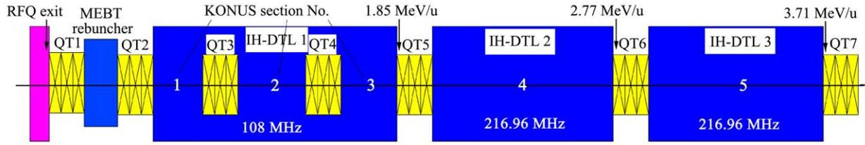
Fig. 1 (color online) Layout of CSR IH-DTL section.
