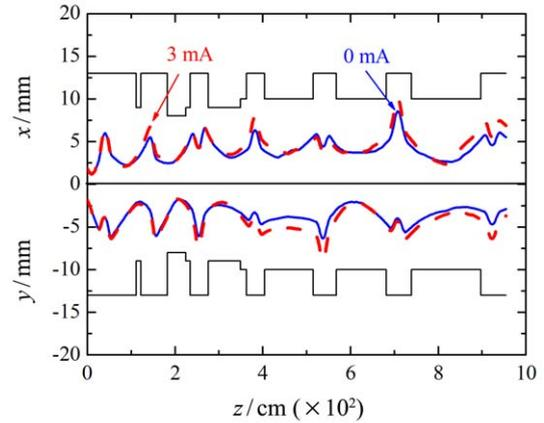
Fig. 10 (color online) Transverse beam envelopes of the CSR-IH-DTL.
