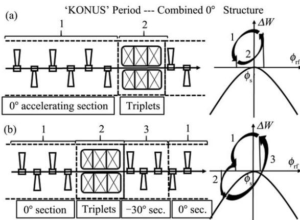
Fig. 2 The KONUS period and the principle of KONUS beam dynamics<sup>[4]</sup>.
