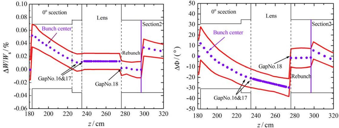
Fig. 5 (color online) The phase envelope and energy spread in the first CSR-IH-DTL cavity and the bunch center motion with respect to the synchronous phase.
