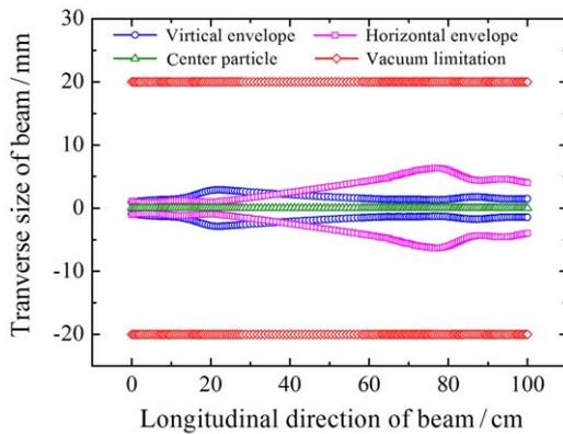
Fig. 3 (color online) The beam envelope of the MEBT.
